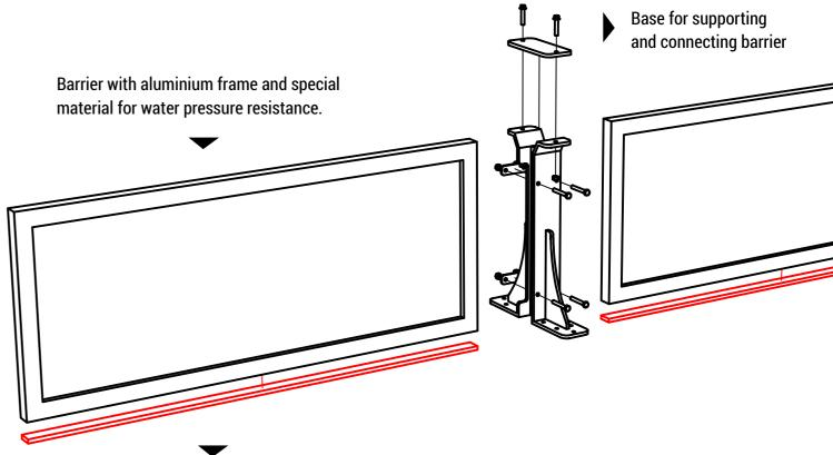
High-strength EPDM rubber all around the barrier to provide better insulation.
