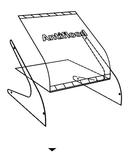
It consists of separate pieces which can be tied together in three points.
