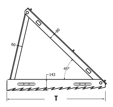
AntiFlood Quick Dam is a heavy duty, modular system, which has been designed by our company to divert flood water. It consists of two foldable stands, three horizontal spacers, a sheet metal cover and can be assembled without tools. The system is designed to occupy minimum storage space.
