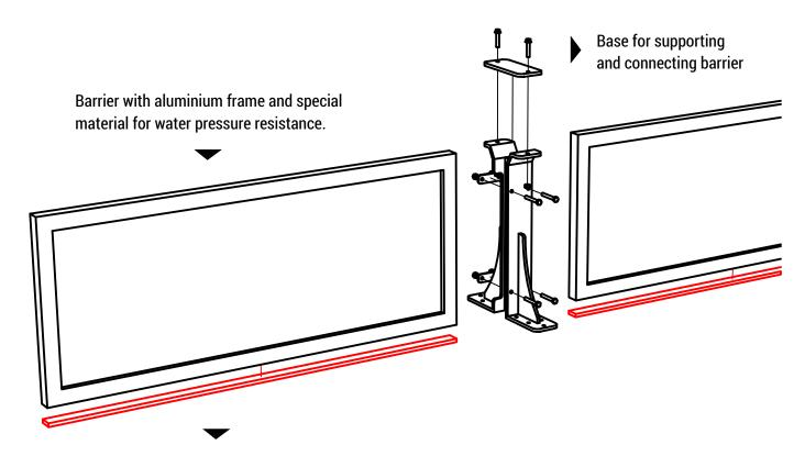
High-strength EPDM rubber all around the barrier to provide better insulation.
