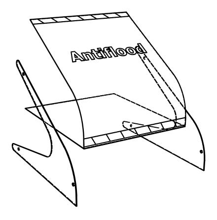
It consists of separate pieces which can be tied together in three points.
